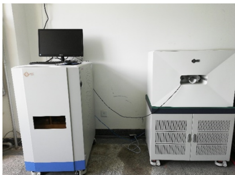
图3 MesoMR23-060H-I 核磁共振成像分析仪 Fig.3 MesoMR23-060H-I magnetic resonance imaging analyzer
